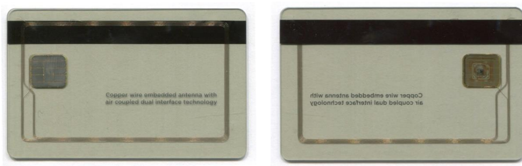
Figure 7. Dual-Interface Card Samples with Full Perimeter Embedded Copper Wire Antenna
