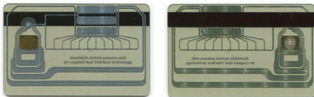
Figure 5. Dual-Interface Card Sample with Aluminum-Etched Antenna
