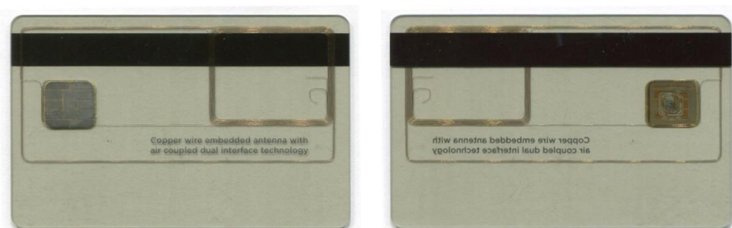
Figure 6. Dual-Interface Card Sample with 3/4-Size Embedded Copper Wire Antenna
